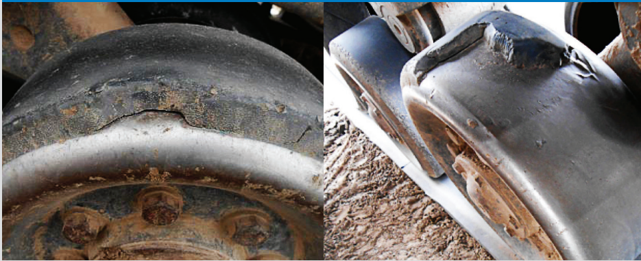
Major damage to outer surface and significant separation from the metal hubs.
